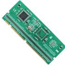
Fig. 14. PIC24FJ96GA010 mounted on an MCU card.
